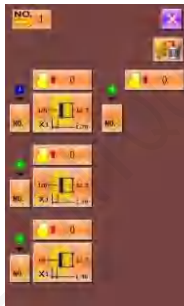
The right figure is the edition on the data of the continuous stitching. On specific operation, please refer to Continuous Sewing Data Input
