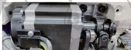
Stepper Motor Driven Thread Trimming & Presser Foot Lifting
