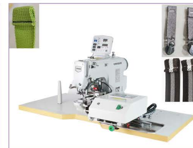
UN430D-ATF Electronic ribbon belt folding and bartacking machine
