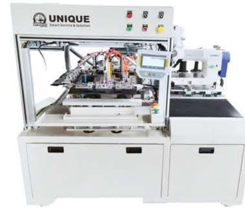
UN-3AC Fully automatic three-clip collar sewing and cutting machine
