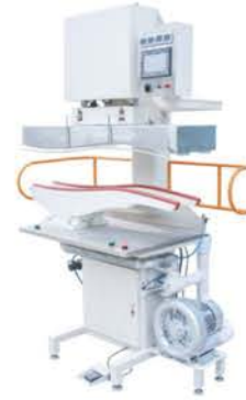
UN-8402P Automatic sleeve side seam press
