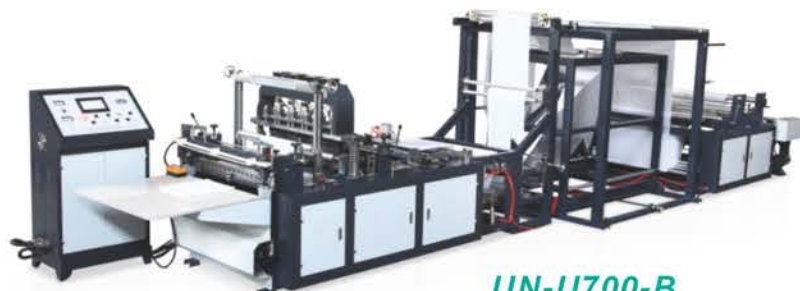
UN-U700-B Nonwoven bag making machine Working area: Length: 200-600mm Width: 100-800mm
