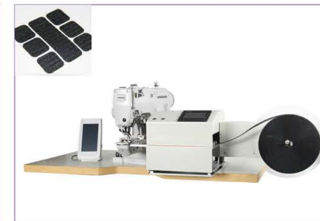
UN436D-AVCB Automatic velcro tape cutting and attaching machine with bottom feed with max. tape size 9*6cm UN342G-AVCB with max. tape size 30*20cm UN326G-AVCB with max. tape size 20*10cm UN430D-AVCB with max. tape size 4*3cm
