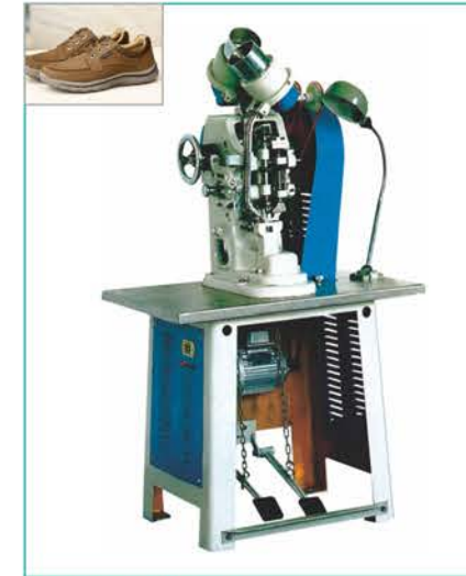
UN-EH-95 Automatic electric double side eyelet punching machine
