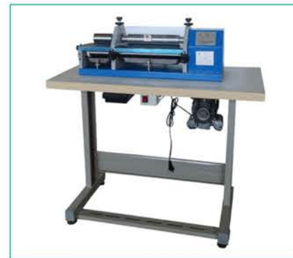
UN-WG107 White gluing machine (2 gluing areas) UN-WG107 width: right 100mm, left 270mm iron roller
