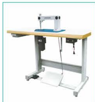
UN-FT669 Seam opening and tape attaching machine
