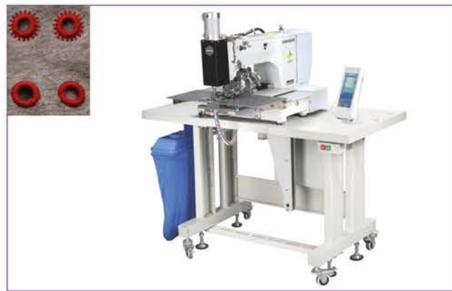
UN2210-20 Electronic eyelet hole punching and sewing machine Max hole diameter 6mm
