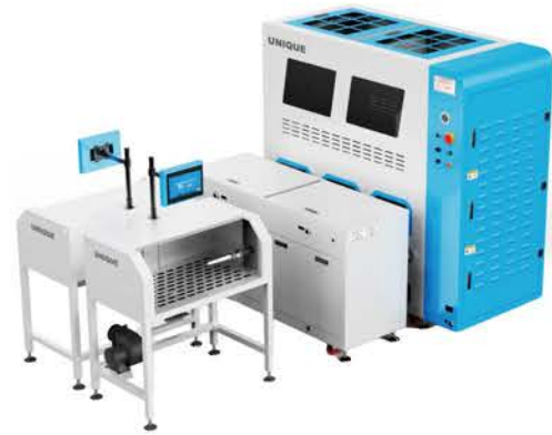
UN8208R High-precision intelligent down & cotton filling machine UN8208R 2 filling port & 8 scales UN8416R 4 filling port & 16 scales
