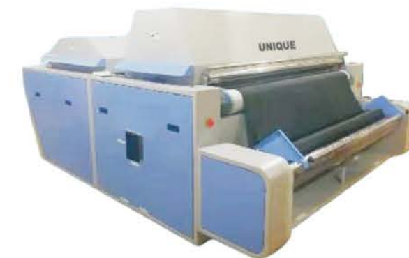
UN-FS2700-72 Fabric shrinking and forming machine (working width 2200mm) UN-FS2700-72 working width 1800mm UN-FS2700-88 working width 2200mm
