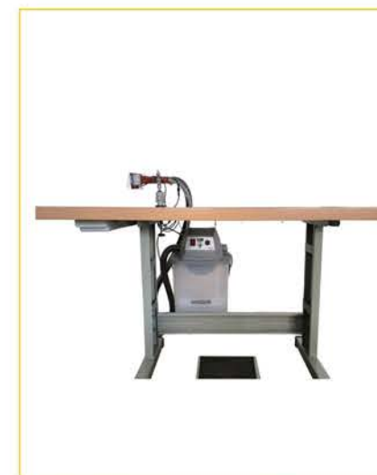
UN-TX-2022T Thread trimming machine with sensor with brushless motor
