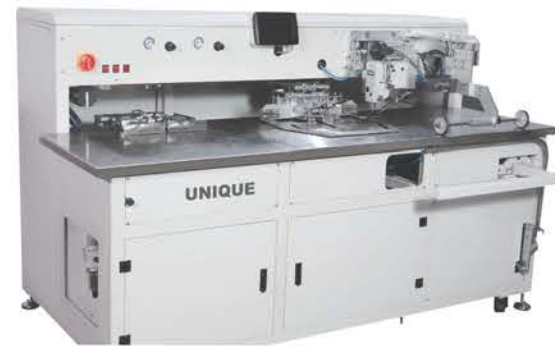
UN-163-TD Automatic pocket setter for kangaroo pocket With size of 50*30cm
