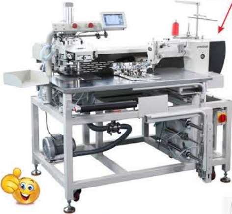
UN-720-TD Automatic pocket folding and setting machine (iron free)
