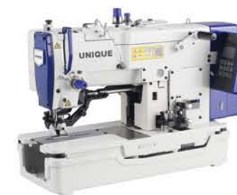
UN781N-2S Direct drive straight button holing machine with 2 step motors 1 step motor for auto foot lifter and the another for silent and non-stop button hole cutting. UN781N-1S With only 1 step motor for foot lifter
