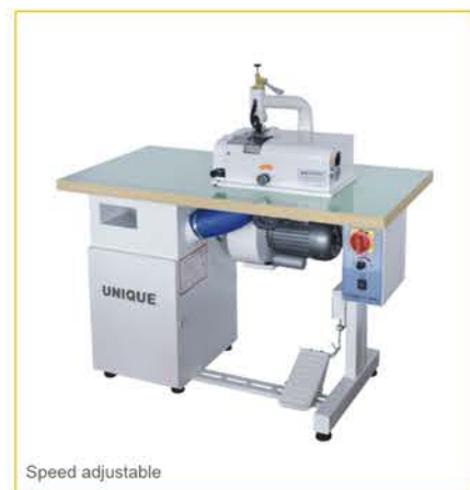
SK-1923 Leather skiving machine with trash suction device
