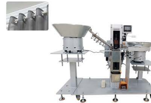
UN-RA98F Automatic curtain ring attaching machine
