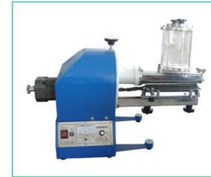
UN-G250 Yellow glue machine Glue width: 0-230mm
