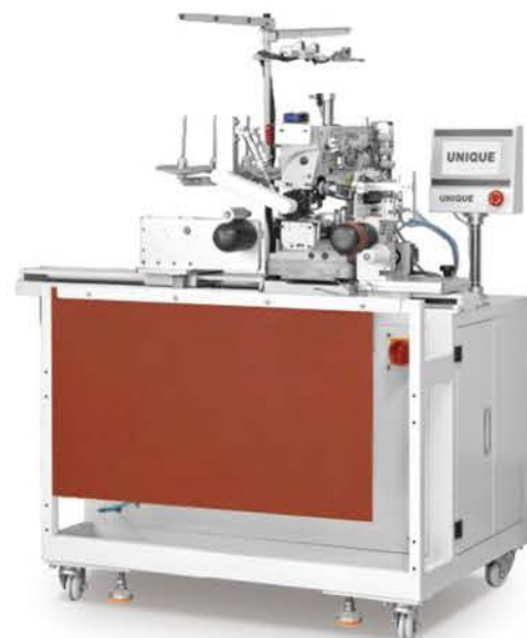
GK-346-2 Automatic elastic waistband attaching machine
