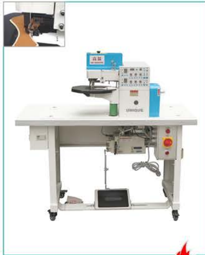
UN-CM292 Computerized hot-cement edge folding machine
