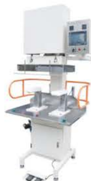
UN-8403 Sleeve placket press-double head
