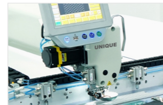
Electronic follower foot prevents thread skipping and thread breakage
