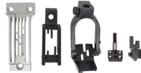
B926-8A针位/Needle gauge
