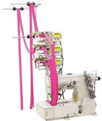
同步送带装置(送带装置通用性) Synchronous tape feeder(Generality of tape feeders)
